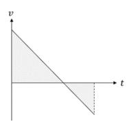
Gradient of graph: acceleration,  $ms^{-2}$  Area under graph: displacement, m
