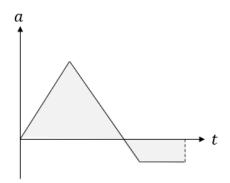
Gradient of graph: jerk,  $ms^{-3}$ Area under graph: velocity, v
