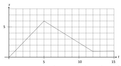
Given the displacement time graph above, find the velocity function for time  $5 \le t \le 12$ . Hence, find the acceleration from t=6 s to t=10 s.
